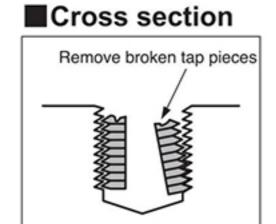
•To remove a broken tap end that is stuck in a hole, make a hole in its center using an electrode of one-half the diameter of the tap.
